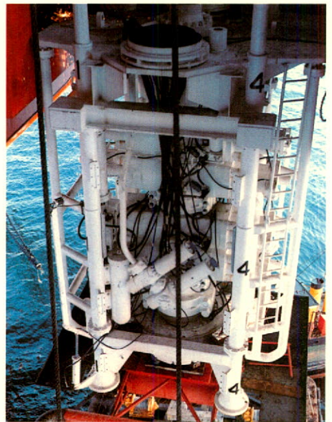
The BVRS offshore drilling fleet is equipped with very sophisticated technical and mechanical equipment such as the blowout prevention system above.
