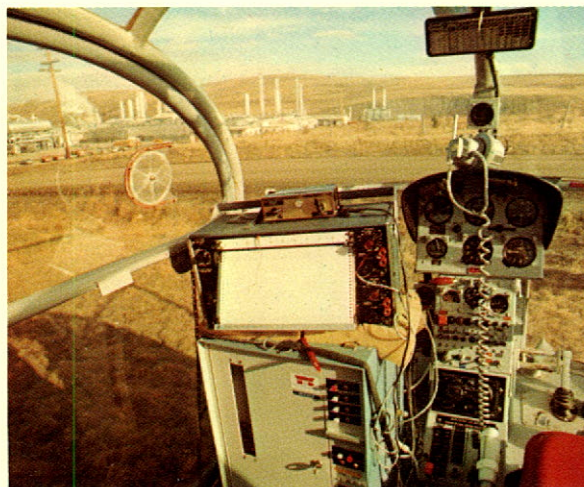
Western Research and Development airborne pollution monitoring equipment.
