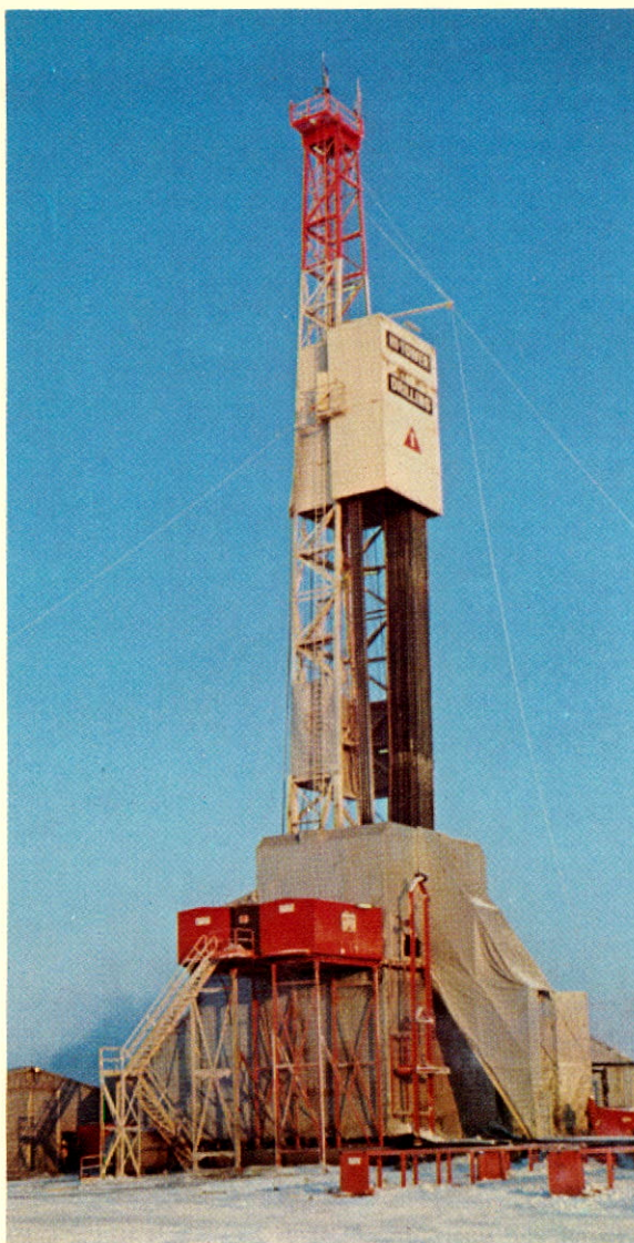
Hi-Tower's new 20,000 foot Hercules Transportable Rig, Delta #1 at work on Hooper Island in the Mackenzie Delta.
