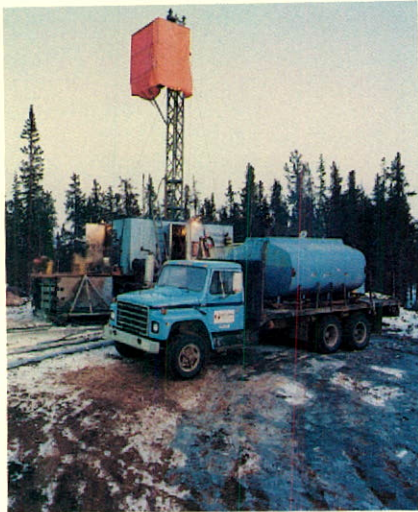
Surface diamond drill coring
