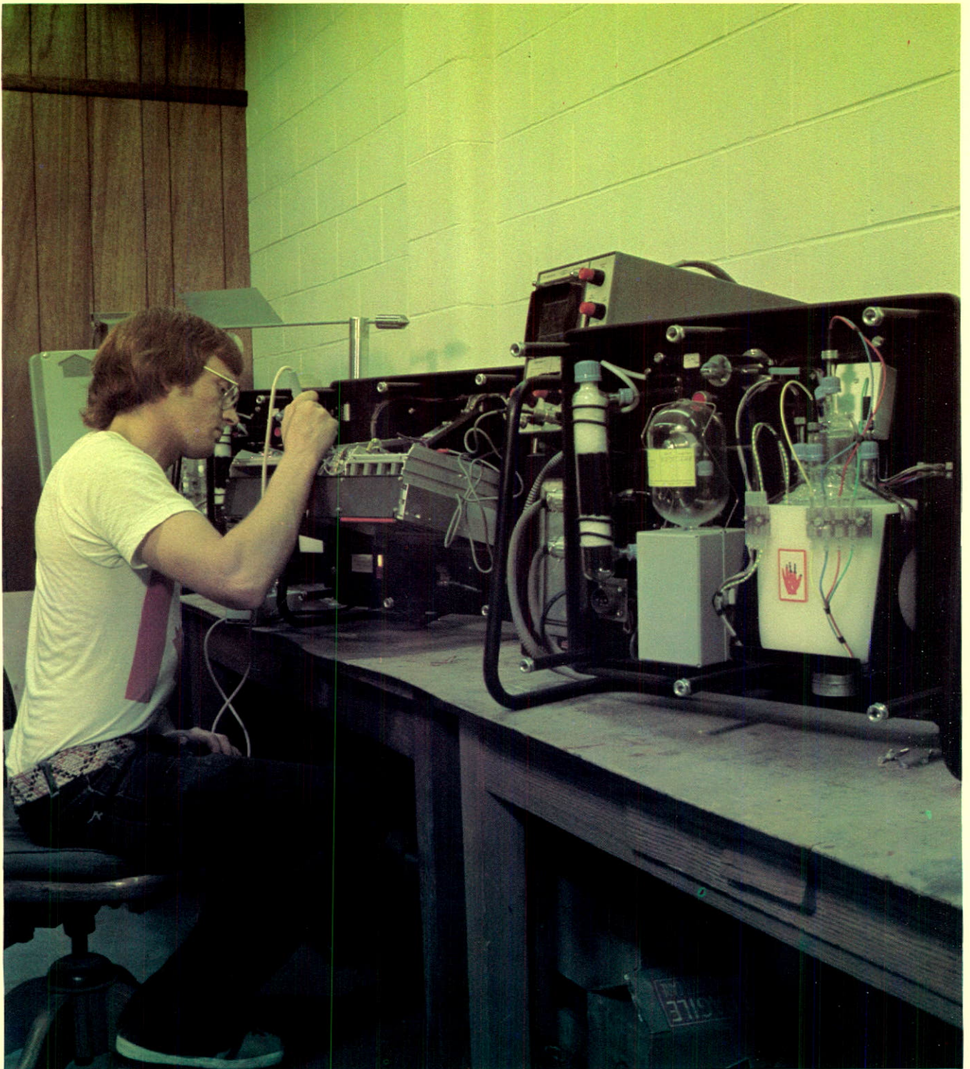
Servicing of sulphur dioxide air monitoring instrument.
