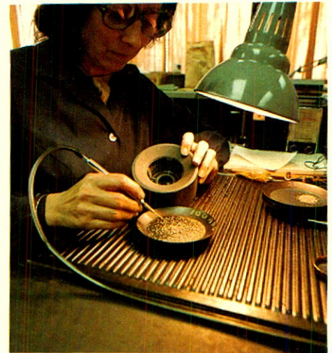
Inserting industrial diamonds in a core hole drilling bit in Bow Valley's Vancouver plant.
