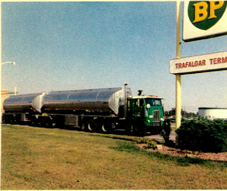
This newly-developed delivery vehicle for light fuels is known as a "B Train". Designed for improved stability, it features a special coupling between the two trailers.
