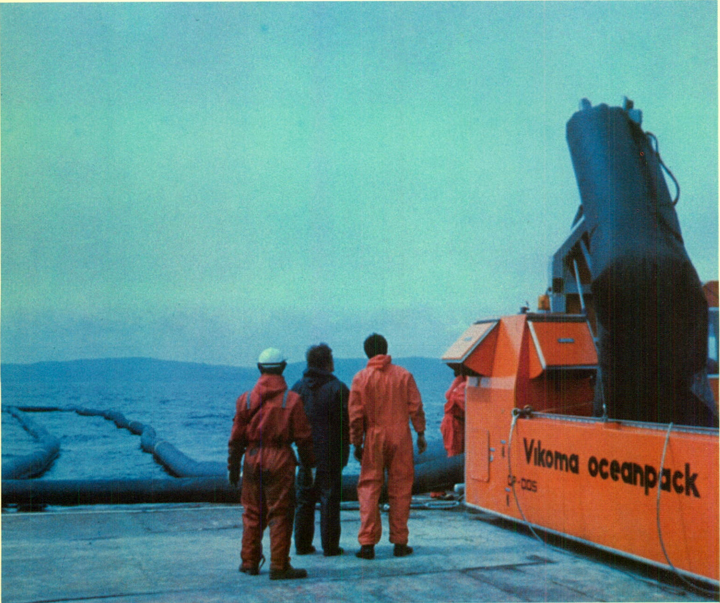
Deploying the Vikoma boom, designed by BP for oilspill containment, during an exercise off Botwood, Newfoundland.
