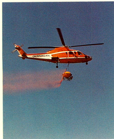
Helicopters were used in 1982 in tests of BP dispersants for potential use on marine oil spills.
