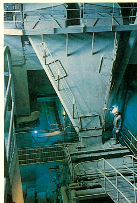
Crushing of raw materials in a hammermill... the first stage in the cement manufacturing process.
