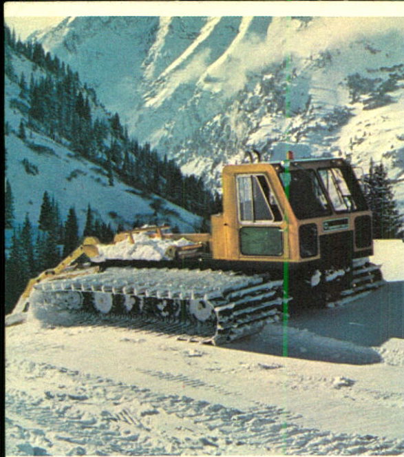
The Skidozer 501 trail groomer is designed for the maintenance of ski slopes.
