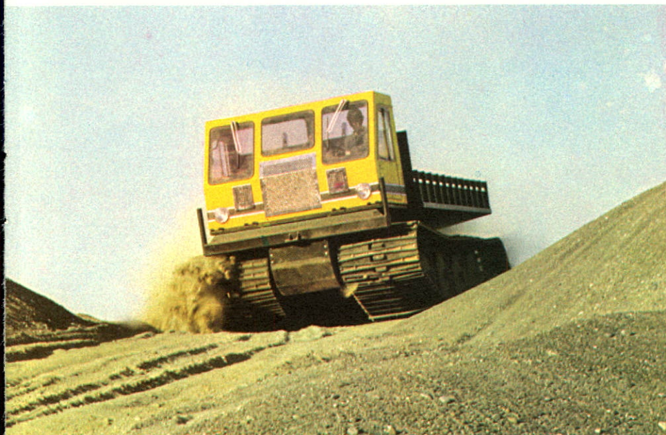
The MTT Muskeg carrier. The largest carrier manufactured to date by the Industrial Division, this all season, all terrain vehicle has a carrying capacity of 30,000 pounds.
