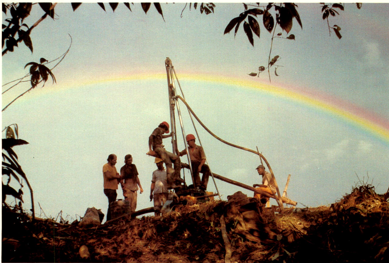
Drilling shot holes for seismic survey, Quibdo, Colombia.
