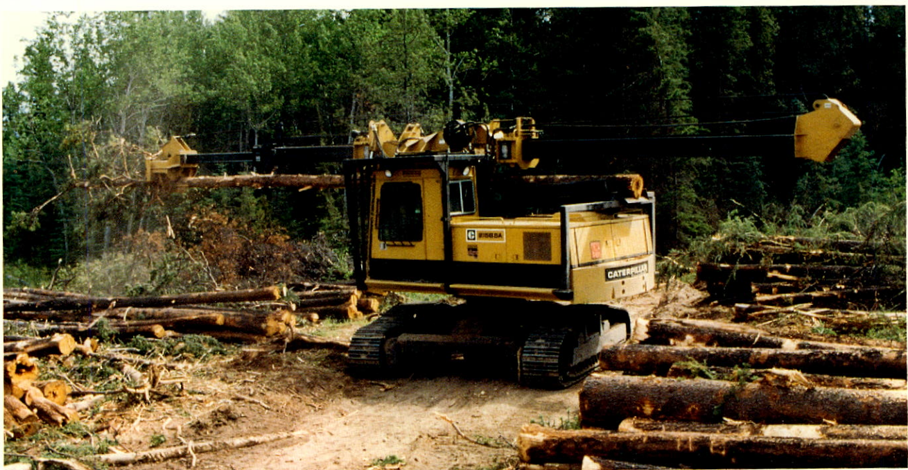
Caterpillar delimeter removes branches and cuts trees to specified length in one easy operation.
