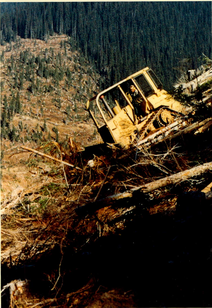
Four new tractors made their debut, incorporating the elevated sprocket design proven on larger models. This 90 horsepower D4H tractor handles steep slopes easily in Kootenay logging operation.
