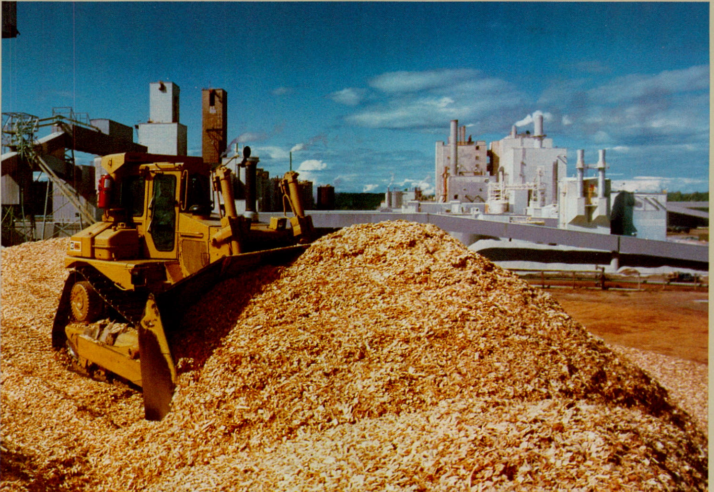
This 335 horsepower Cat D8L Tractor pushes 45 cubic yards of wood chips at one time. Several D8Ls work at pulp mills throughout the province.
