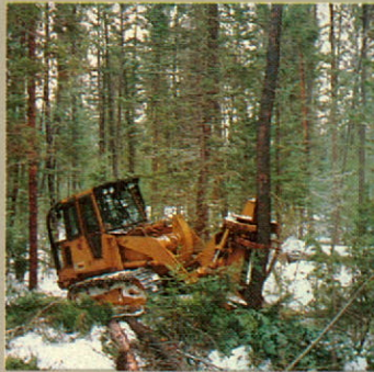
Mid-size track loader with cutting head made its debut in Interior forests.
