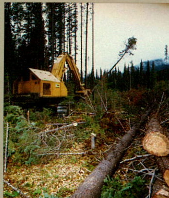
Cat 227 Logger, which fells and bunches trees, is a familiar sight in Interior woods.
