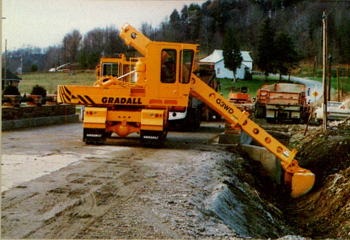
Gradall hydraulic excavators, identified by their telescoping boom, are suited to many specialty jobs.
