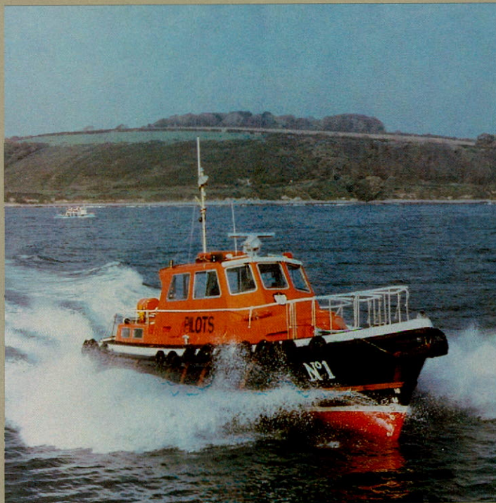
This 56-foot, Caterpillar-powered craft ferries pilots to ships entering port of Falmouth, Cornwall.
