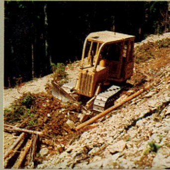
Custom version of Cat's smallest tractor, the D3B, handles utility jobs for East Kootenay logger.
