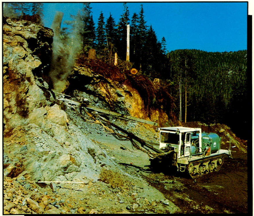
Familiar machine in building logging roads, Finning-designed pneumatic Tank Drill moves rock on Vancouver Island.
