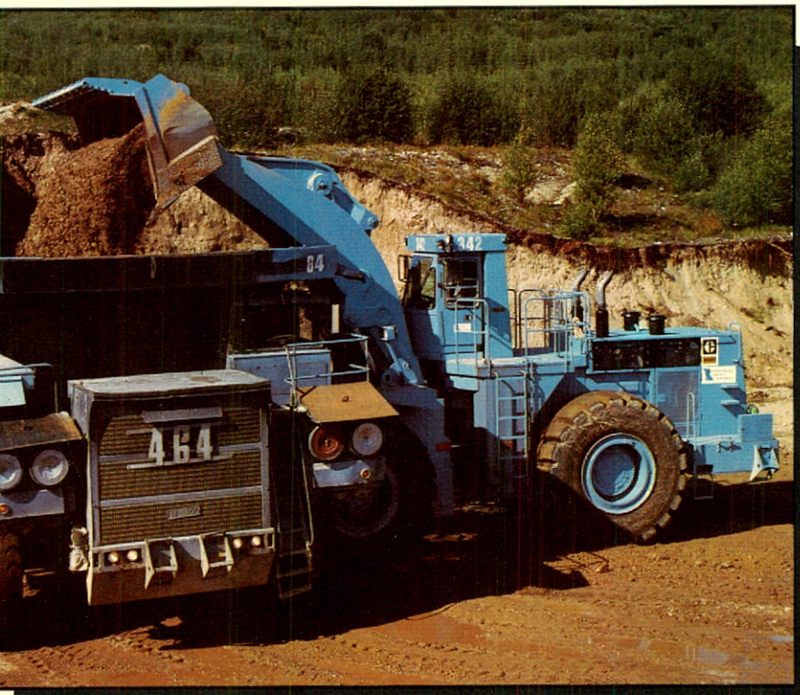
High lift design gives Cat 992C wheel loader ability to load larger trucks at copper mine in the Highland Valley.
