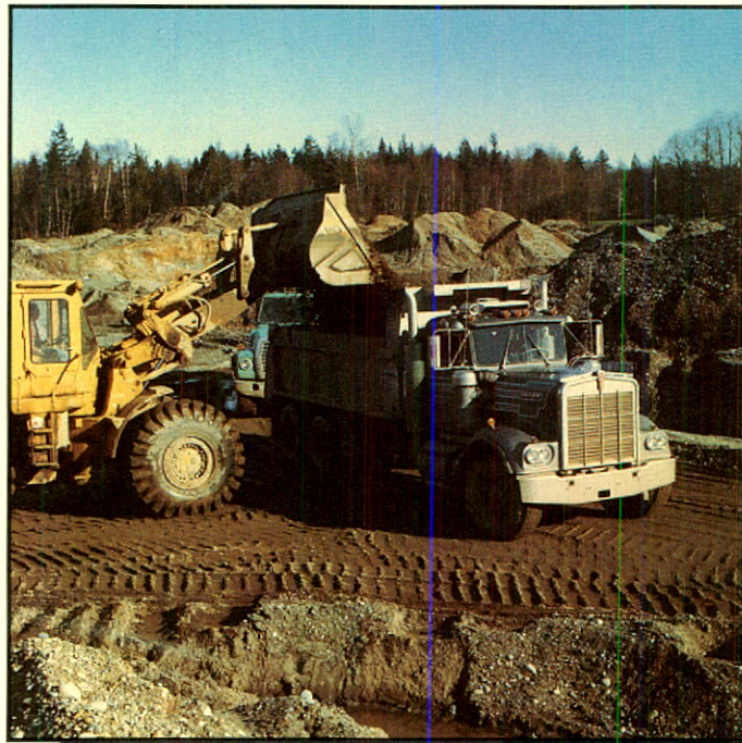
Caterpillar products dominate Fraser Valley gravel pit when Cat 980 wheel loader fills Cat-powered truck.
