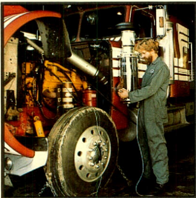
Power analysis tool diagnoses truck engine performance.
