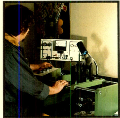
Sophisticated test unit measures balance of rebuilt turbocharger.
