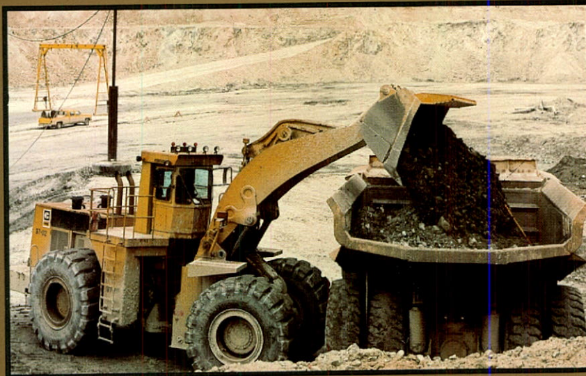
Extended reach on "High Lift" version of largest Cat loader, the 992, allows loading of 110 tonne (120-ton) trucks in open pit mining.
