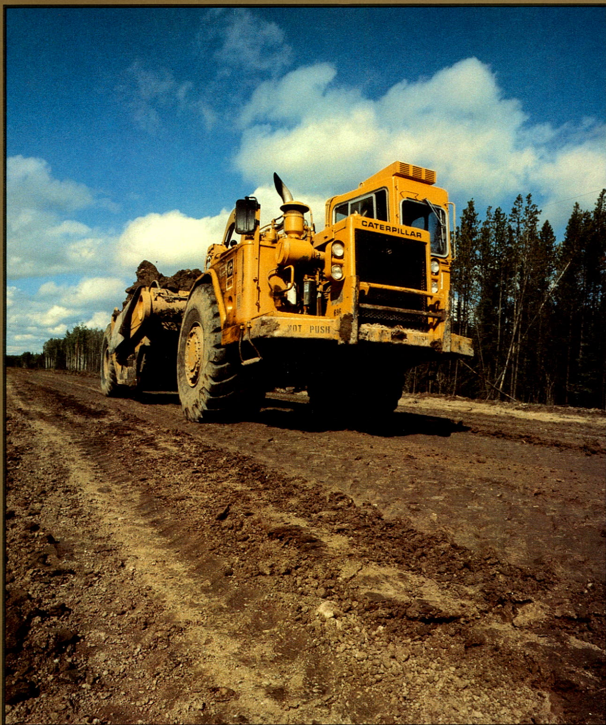
Initial development of northeast coal project makes work for Caterpillar 621B scraper building access road to new town of Tumbler Ridge.
