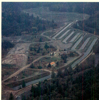
Little Qualicum Spawning Channel completed in 1979. Artificial spawning channels successfully provide optimum spawning and rearing conditions for salmon. (A. Lill)
