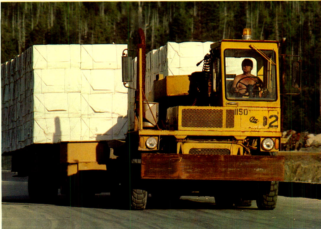
An Ottawa pulp carrier moves a load of baled pulp to the deep water dock of CanCel's Skeena Pulp division at Prince Rupert.
