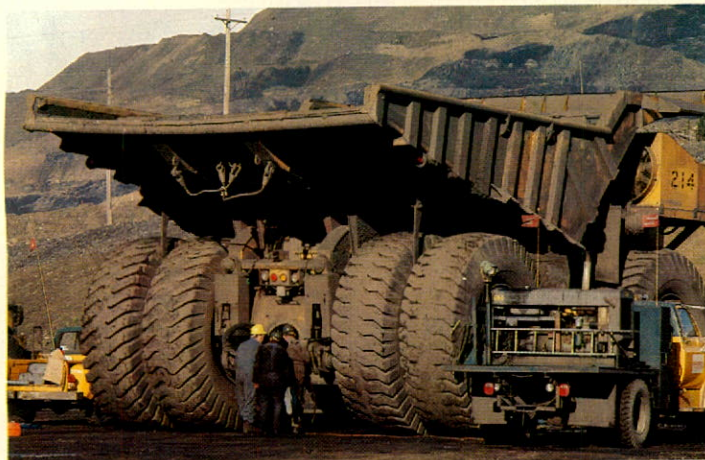
One of a fleet of 180 tonne trucks used for hauling rock from the open pit.
