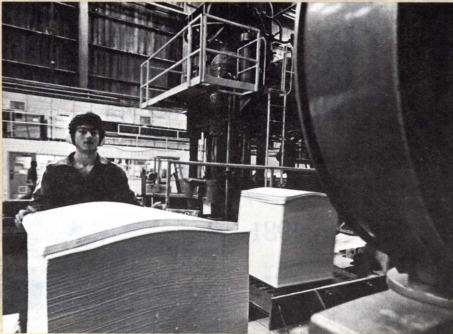
Sheets of air dried pulp are automatically cut and stacked at Skeena Pulp division. Each stack is then weighed by Eric DeJong to ensure accuracy before it is baled and wrapped for shipping.
