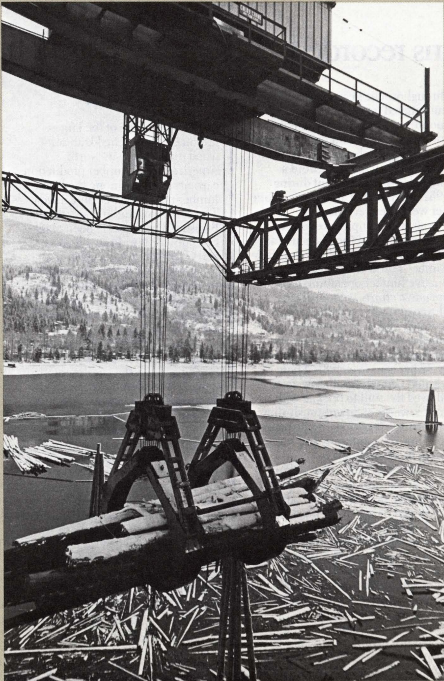
Wood chips for the pulping process at the Celgar Pulp mill in Castlegar are made from logs like these being plucked from the river by the Colby crane. Despite deteriorating world pulp prices, Celgar Pulp operated at full capacity for most of 1982 because of its high efficiency.
