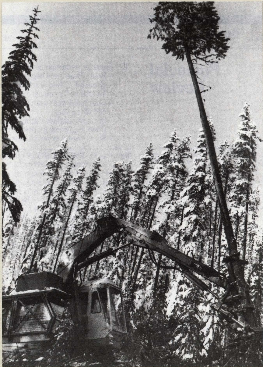
Mechanical harvesting machine used in company-managed forests near Vanderhoof, B.C. ensures safe working conditions for woodlands crews and reduces the cost of lumber produced at the nearby sawmill. Giant pincers can cut through a tree trunk in a single motion.
