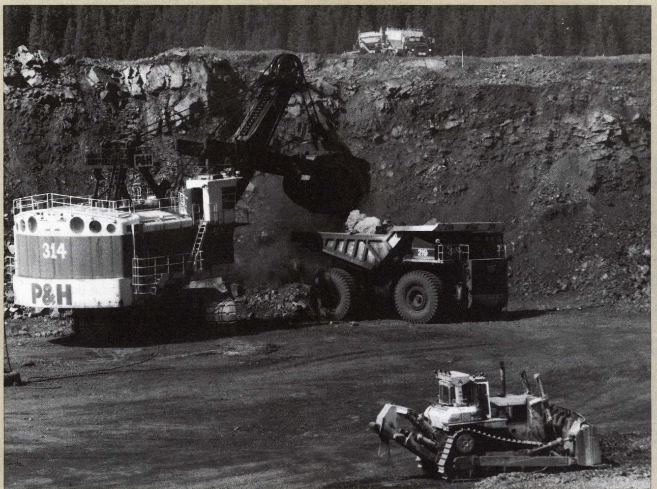
Working in tandem, electric powered shovels and 154-tonne trucks remove the overburden covering the coal seam at Westar Mining's Balmer Mine. During the year, the mine shipped 5.3 million tonnes of coal.
