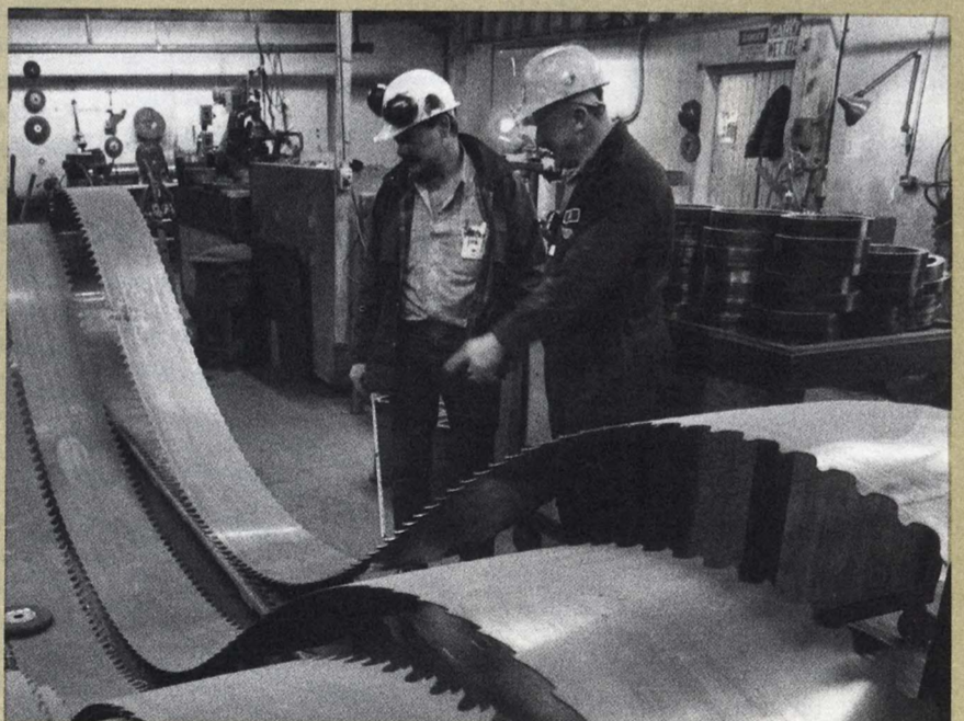
Sharpened to a razor point, these bandsaw blades can be quickly hoisted into position to replace blades dulled by the constant flow of logs along production line.
