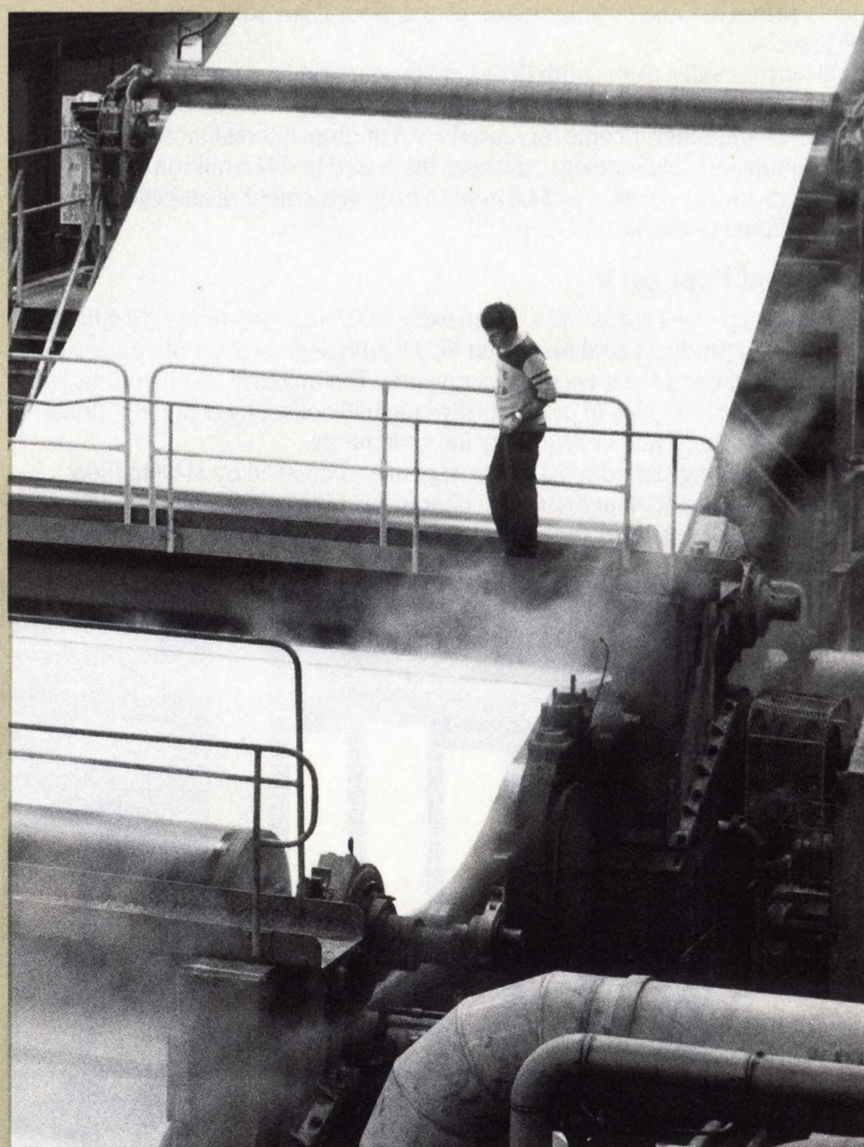
At Celgar Pulp, pulp is formed in a wide sheet before being dried, cut and exported to tissue and fine paper manufacturers around the world.
