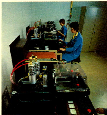
Automated silk screening of circuitry in Hybrid production.
