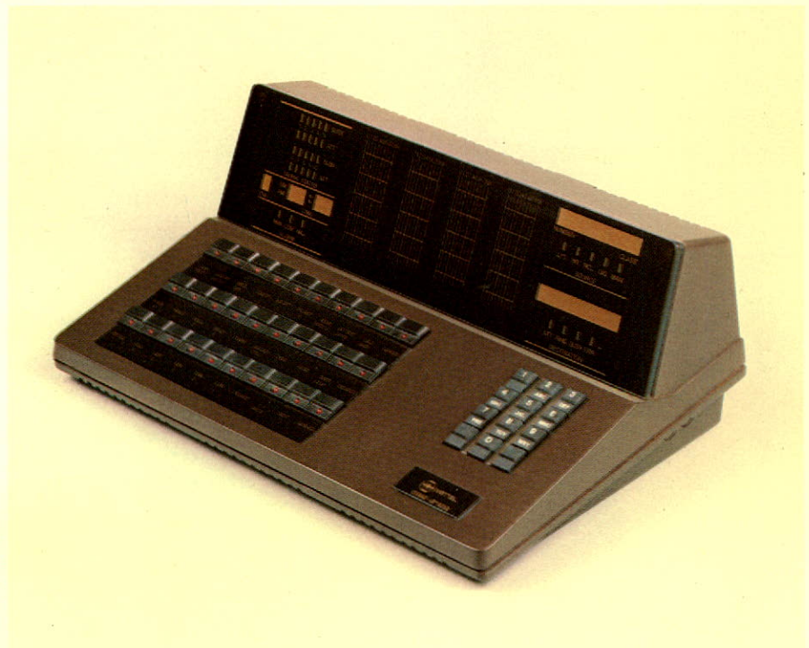
Prototype of a new and restyled attendant console for the SX-200/100 SUPERSWITCH PABX.
