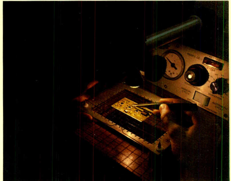
Microscopic inspection of solder contacts in a Thick-Film Hybrid Receiver/Decoder.
