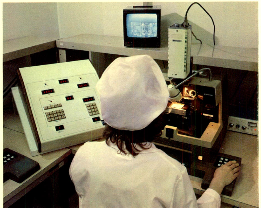
Automated wire bonding station used in the production of integrated circuits.
