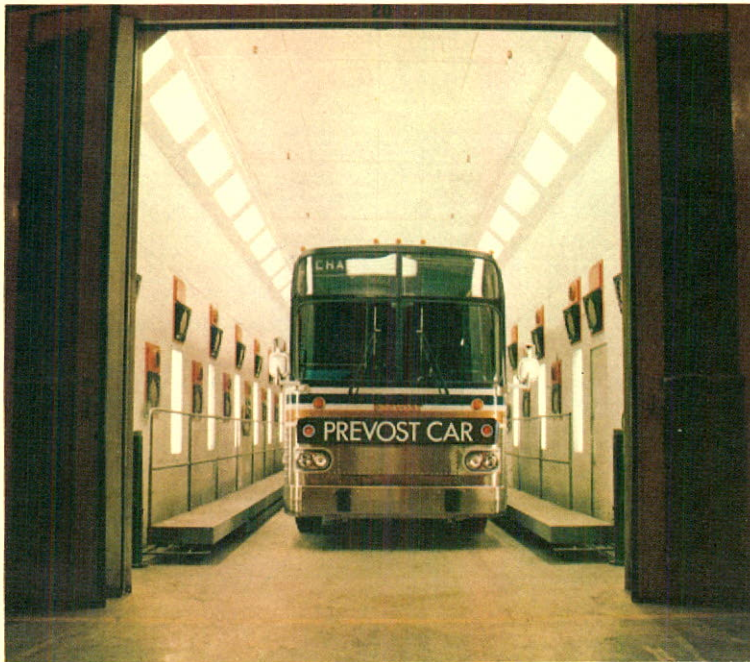
Sunkiss catalytic thermoreactors manufactured by IEC-Holden used as a paint dryer in a new coach plant.
