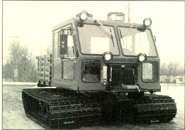
▲ Bombardier Inc., of Valcourt, Quebec, supplied a “Skidoozer” to the U.S. Army through CCC. It’s an all-purpose oversnow vehicle with a capacity for both passengers and cargo.
