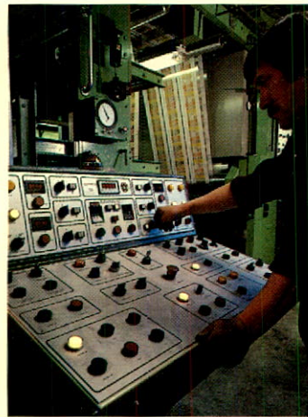
Operations control centre for the new flexographic press designed for high volume production of all types of flexible packaging.
