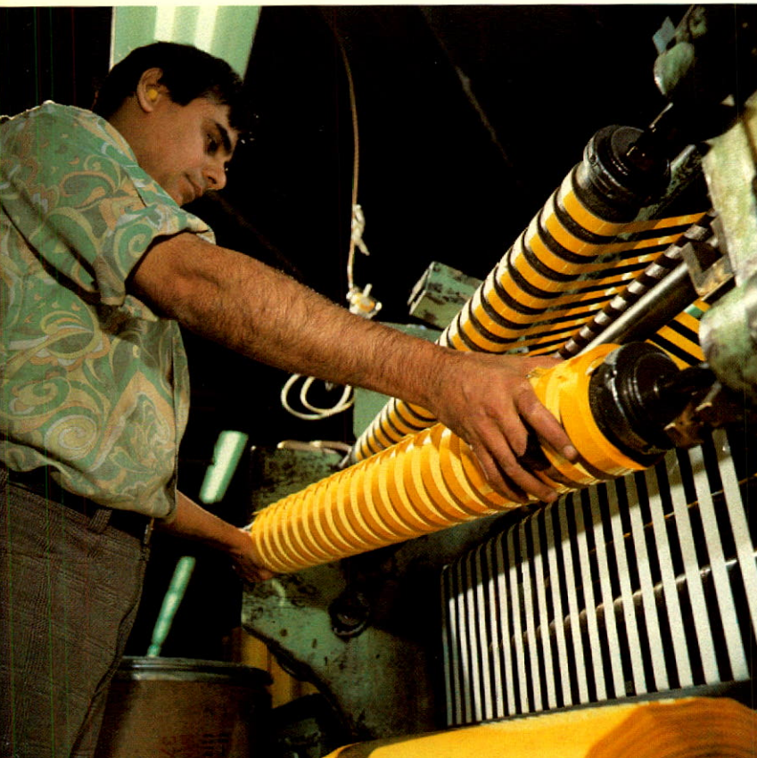
Mansoor Govani takes slitted coils of industrial tape from Beasley French slitting machine which is also used for commercial tapes.
