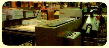
Newly installed equipment provides continuous inline cutting and die cutting from sheeted materials in one operation rather than the several operations needed before.
