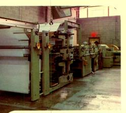
(4) Located at DRG Stationery, Georgetown, the high speed roll-fed, loose-leaf refill machine, capable of running at 1,000 feet per minute, rules, drills, cuts, packages and polywraps in one continuous operation.
