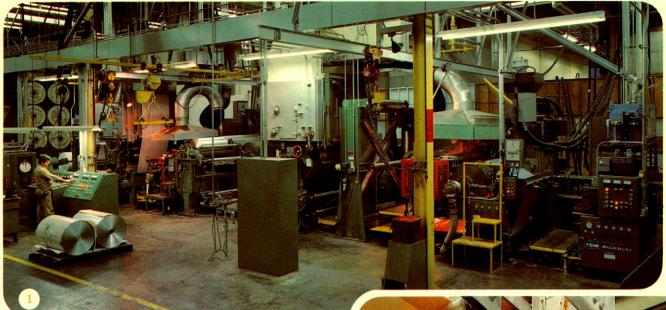
(1) A first in Canada, the tandem coater/laminator developed at DRG extrudes, prints, laminates and coats in one continuous operation.
