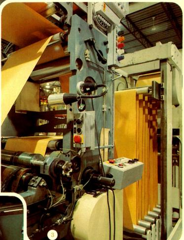
(3) This roll-fed envelope machine for making large open side and open end envelopes is the only one in Canada and more than doubles the capacity of conventional envelope equipment.
