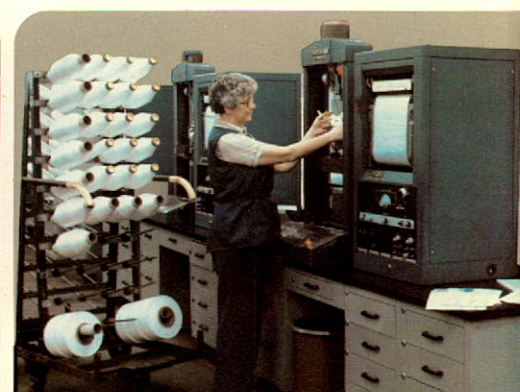
Jessie Hallett, Kingston Works, tests strength of nylon yarn.
