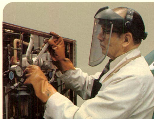
Louis Solc, Research Centre, supplies catalyst to pilot plant in preparation for research on polyethylene resin manufacturing process.
