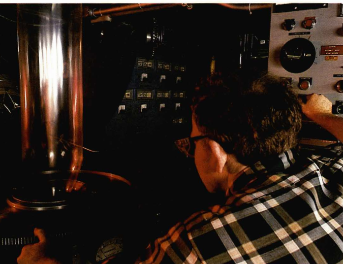
The film line, or bubble, is an important development facility at the Customer Technical Centre. It simulates commercial extrusion of packaging films from polyethylene resins. Technician is Pat McNamee.
