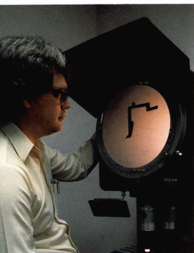
Profile projector, which displays a magnified image, is an extremely versatile design and analytical instrument. Employing it here is technologist Bill Thorne, Customer Technical Centre.
