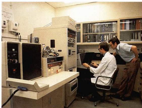
Chemical research requires a variety of sophisticated analytical equipment. Research technologist Peter Gordon, seated, and senior research chemist Dick Dughton, work with an advanced type of gas chromatograph/mass spectrometer. Costing about $250,000, the unit was installed at the Research Centre several months ago.
