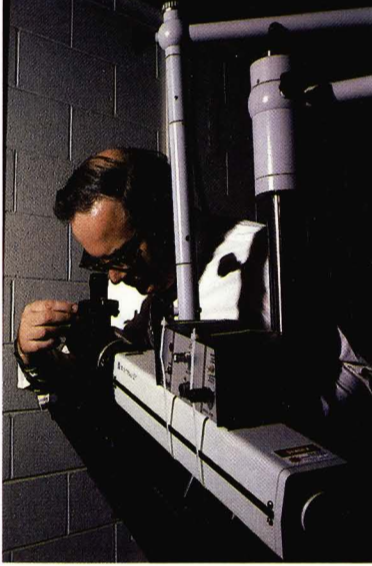
Bruce Robinson and other scientists at the Research Centre, Kingston, employed laser technology to produce this highly accurate speed measuring instrument. This device provides new information on fibre spinning processes and is an important tool for product and process development programs.
