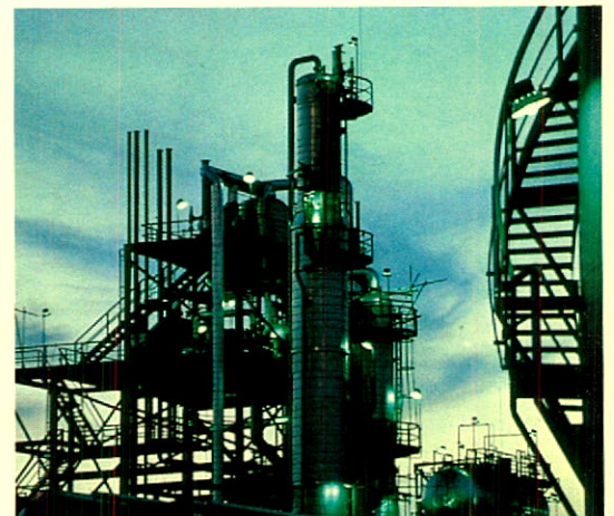
Ethylene oxide plant, Sarnia Division: precursor of ethylene glycol, an essential chemical for antifreeze and synthetic textile fibres.
