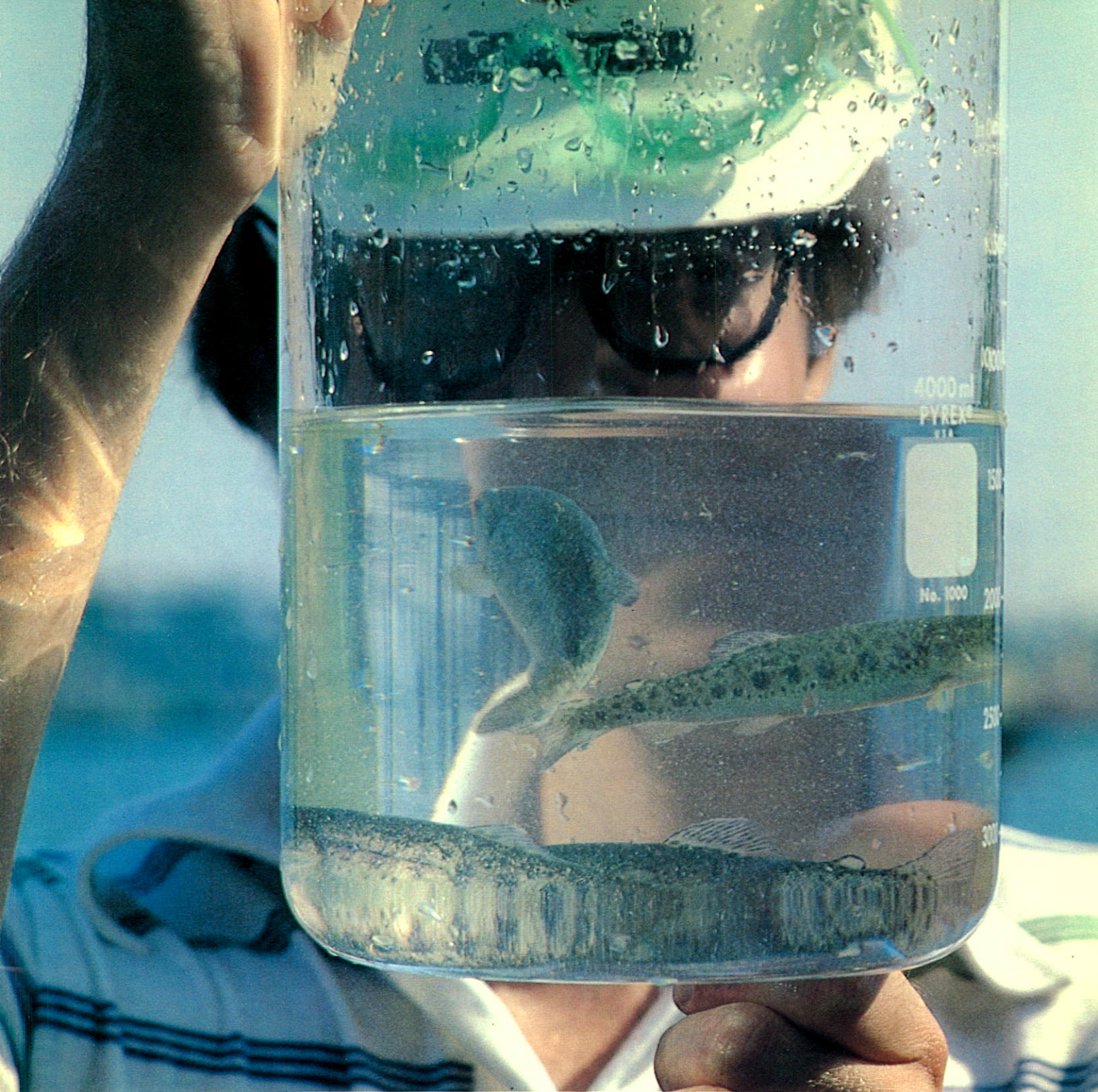
Fingerling trout, a very sensitive species, are used to test effluent water for purity before it is returned to streams, rivers adjoining Dow plants.
