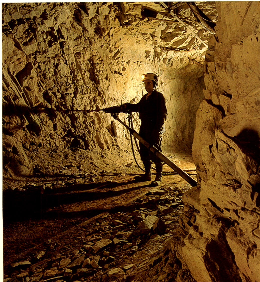
Jack-leg drilling at the Camflo Mine.
