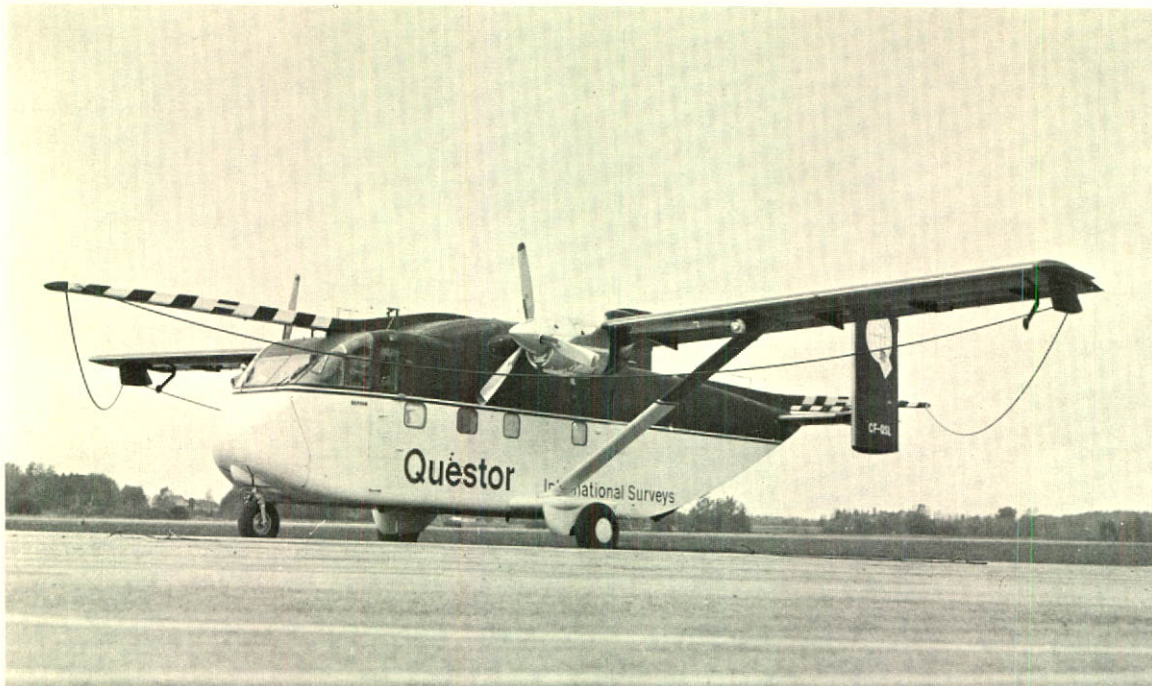
The most recent installation of the Mark VI INPUT System utilizes the Short Brothers STOL Aircraft; using auxiliary fuel tanks, the aircraft can survey the entire day without landing.
