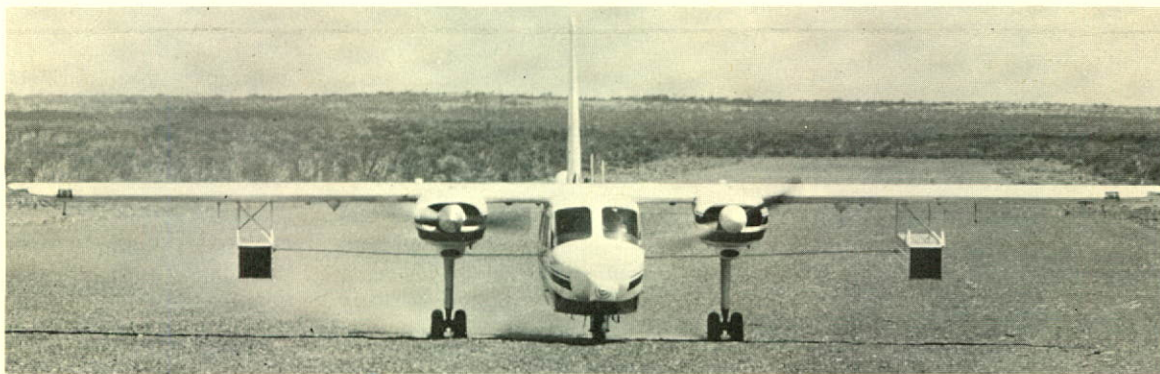
AIRTRACE installation in Britten-Norman Islander aircraft in Australia, air scoops under wings.
