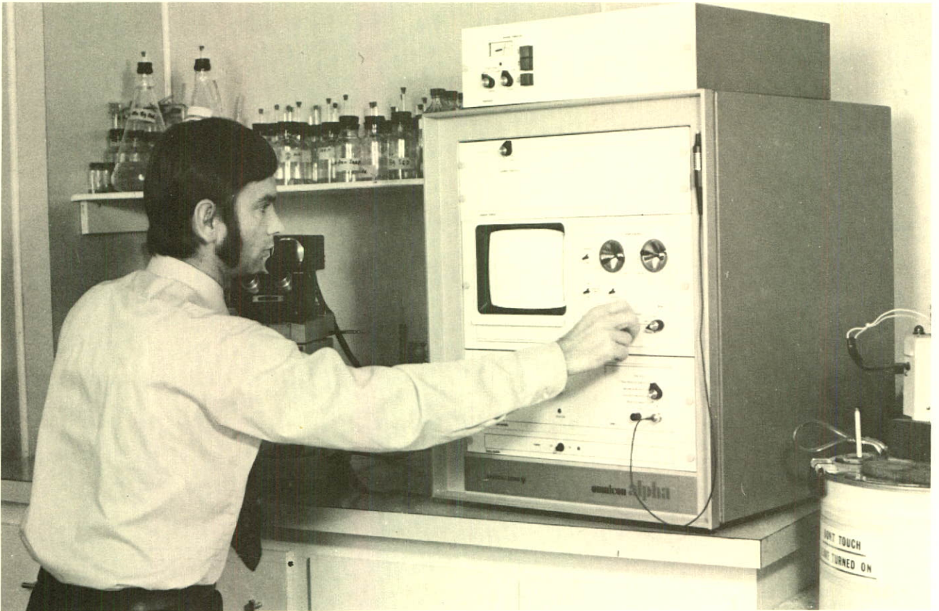
Ludo Daubner, Chief Engineer, testing the optical counter of the AIRTRACE fission track uranium analyser.
