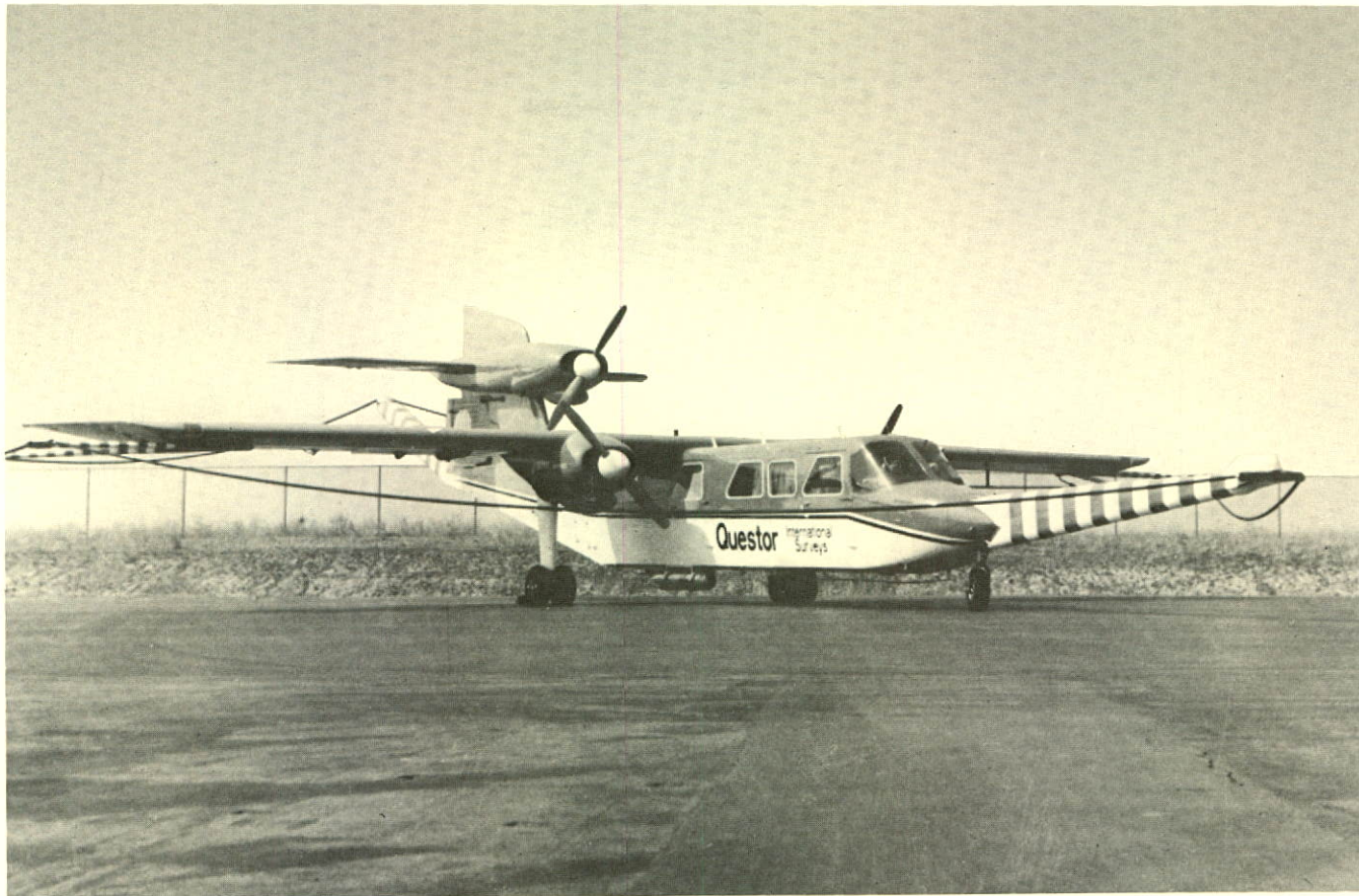
Trislander aircraft equipped with Barringer's INPUT system.
