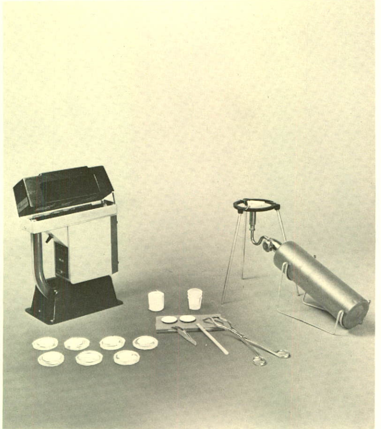
Barringer's Uranium Field Kit, designed for rapid analysis of samples in the field.
