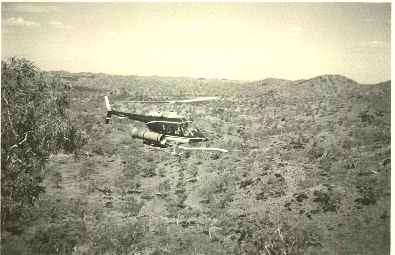
Helicopter equipped with AIRTRACE and Magnetometer on survey in Australia.
