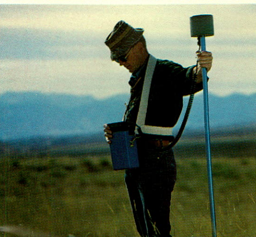
Measuring the Earth's magnetic field during a field survey.
