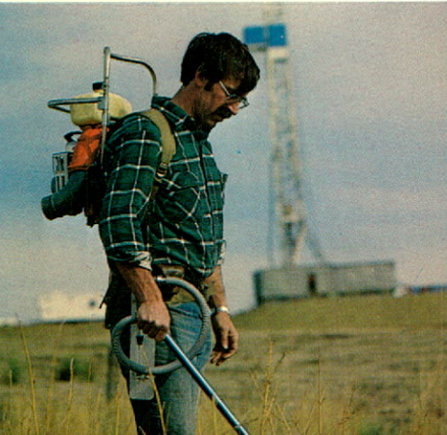
"Sniffing," i.e. taking surface samples for geochemical analyses.
