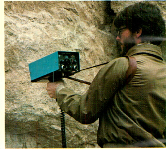
Hand Held Ratioing Radiometer, a new commercial product designed for the spectral identification and classification of clay minerals and the monitoring of vegetation stress.
