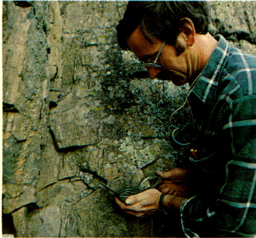
Measuring orientation of fractures in an exposed rock surface.
