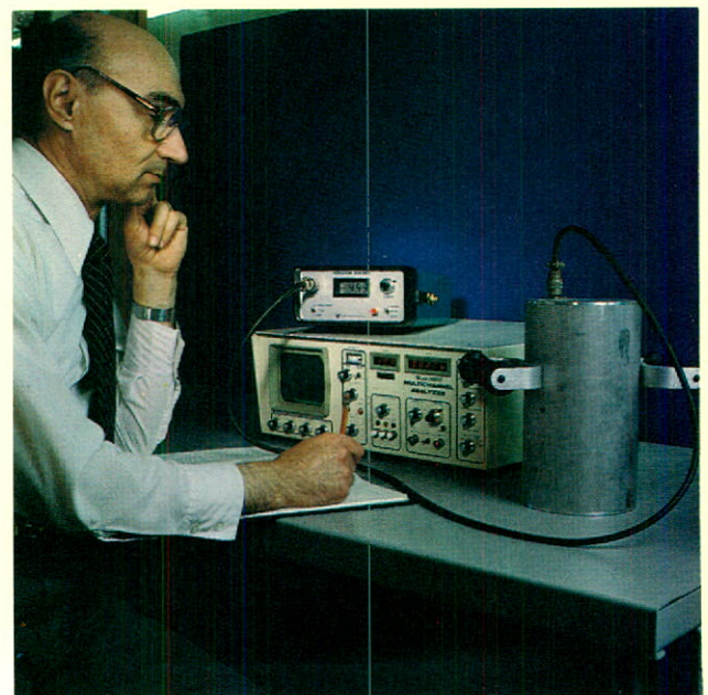
Testing the new potash ore analyzer developed for Saskatchewan Potash Corporation.
