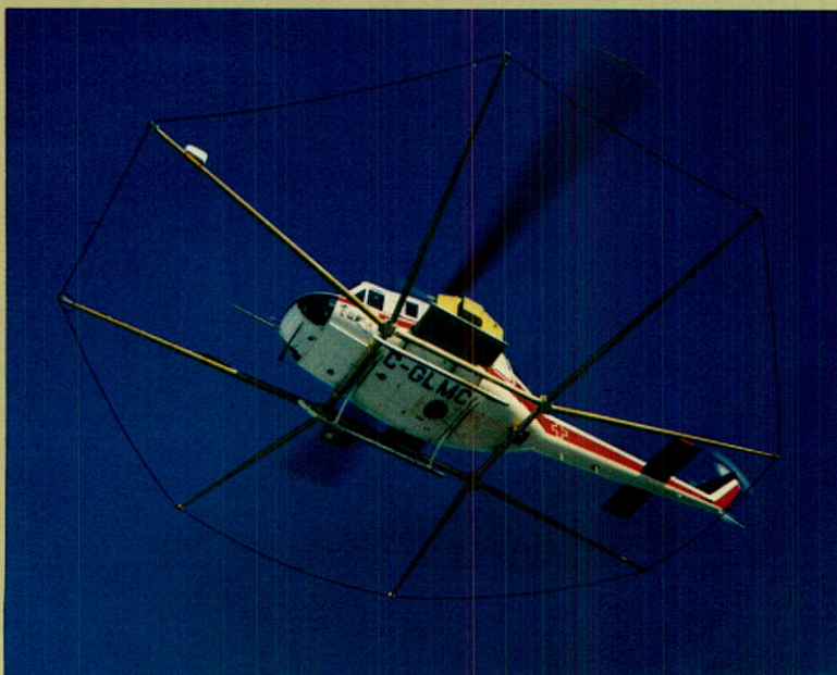
The INPUT system recently installed aboard a helicopter by Questor Surveys Ltd., a Barringer licensee.
