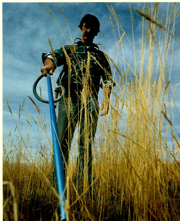
Taking surface samples from geochemical analyses to identify the presence of hydrocarbons.
