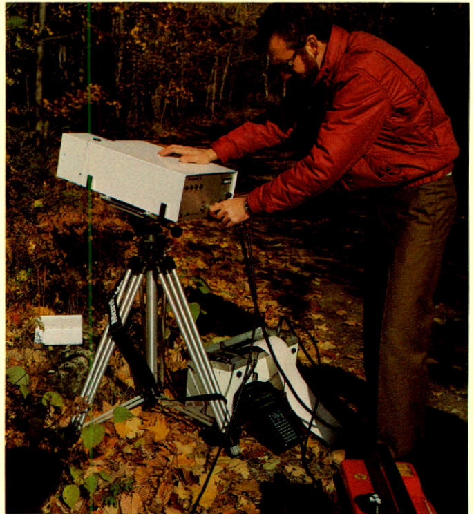
During 1983, Barringer further developed and sold two of its REFSPEC® instruments to the Peoples Republic of China. REFSPEC® measures the detailed reflectance spectra of minerals and vegetation.
