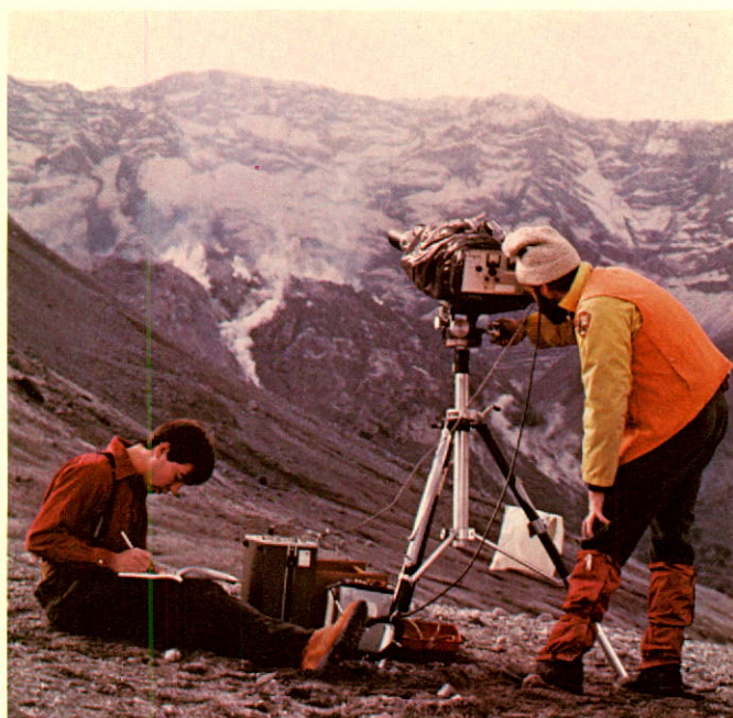
Employees of The United States Geological Survey utilize Barringer's COSPEC to monitor carbon dioxide and sulphur dioxide escaping from Mt. St. Helens. These measurements proved useful in predicting past eruptions from such volcanic activity. (Photo courtesy of The United States Geological Survey.)
