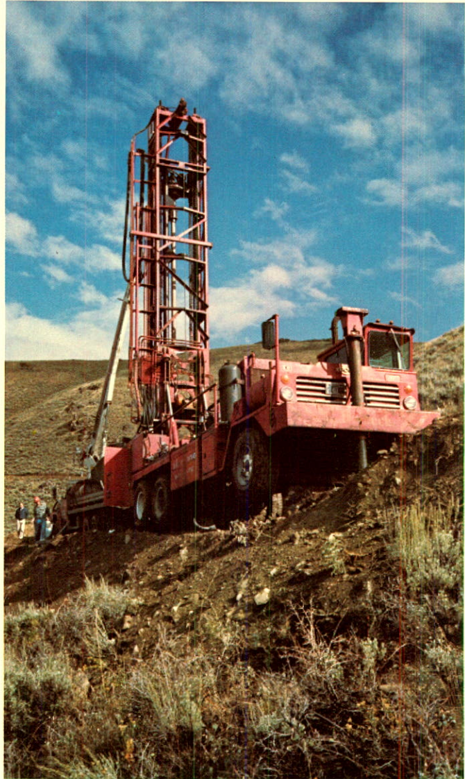
Through its joint venture, Auritech, Barringer drilled 18 test holes in Nevada in 1983 to confirm the presence of precious metals located by various geochemical and geological exploration techniques.
