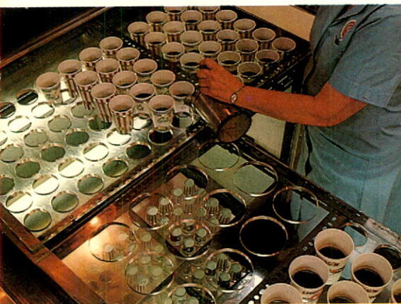
Real coffee, boiling hot, is used for routine quality assurance testing of bondware, at Plant 10, New Toronto.
