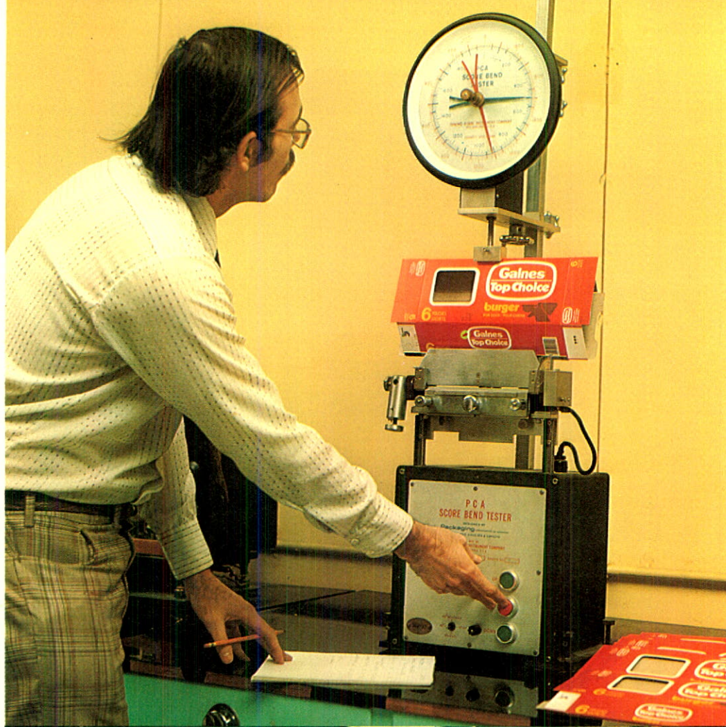
Quality test is performed on folding carton sample by William Kerr, Senior Lab. Assistant at 530 Mount Dennis.
