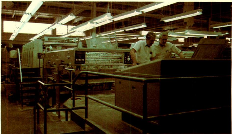
General view of 6 Colour 60" Harris Litho Press installed last fall at Plant 530 Mount Dennis, Ontario. Operator adjusts ink flow from remote push-button stations and ink settings are displayed on centre screen. Continental is Canada's largest manufacturer of folding cartons.
