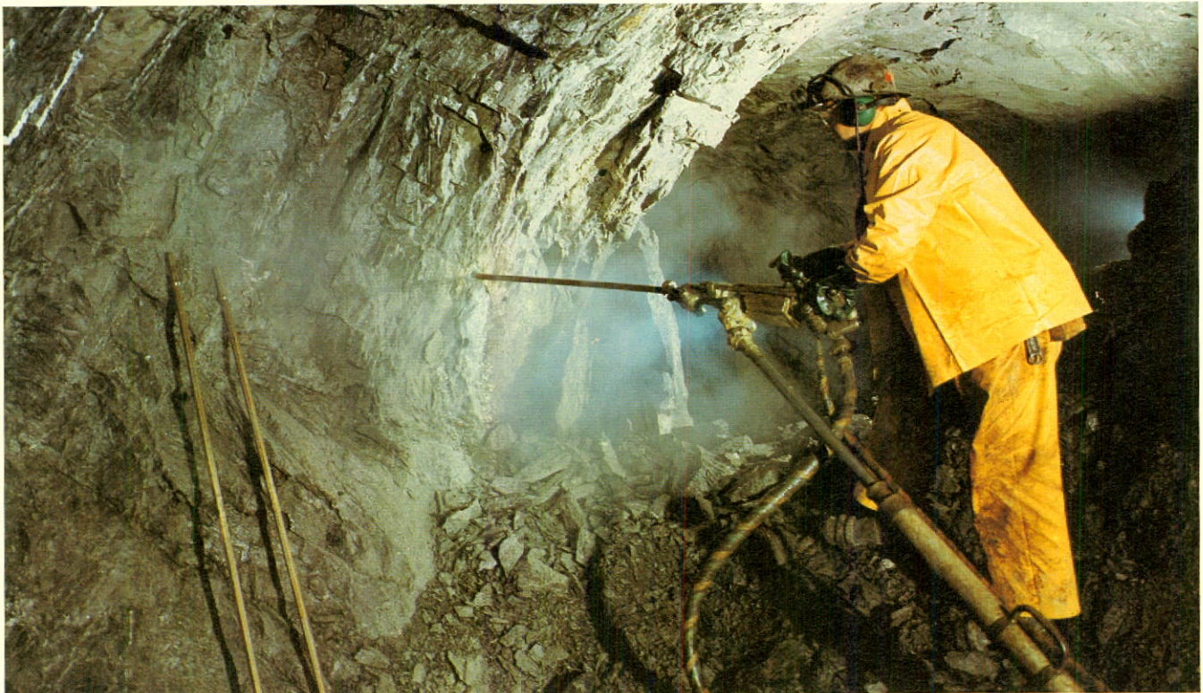
Miner operating an air-leg drill underground.
