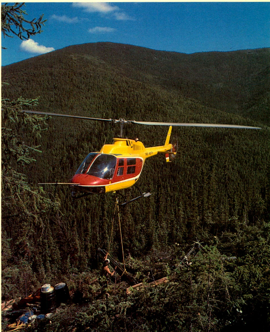
Airlifting Diamond Drill equipment — Yukon.
