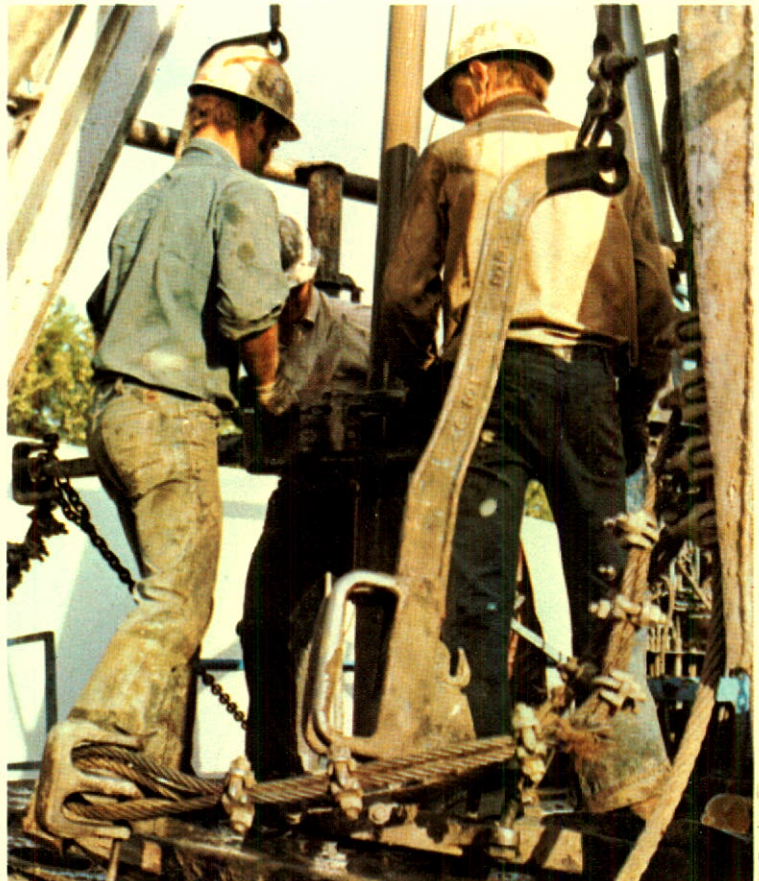
Running production casing — Pennant Venture development well location.
