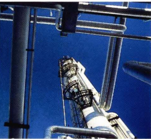
This natural gas extraction plant near Empress, Alberta, can process as much as 56 million cubic metres of gas a day to extract ethane and liquefied petroleum gases.
