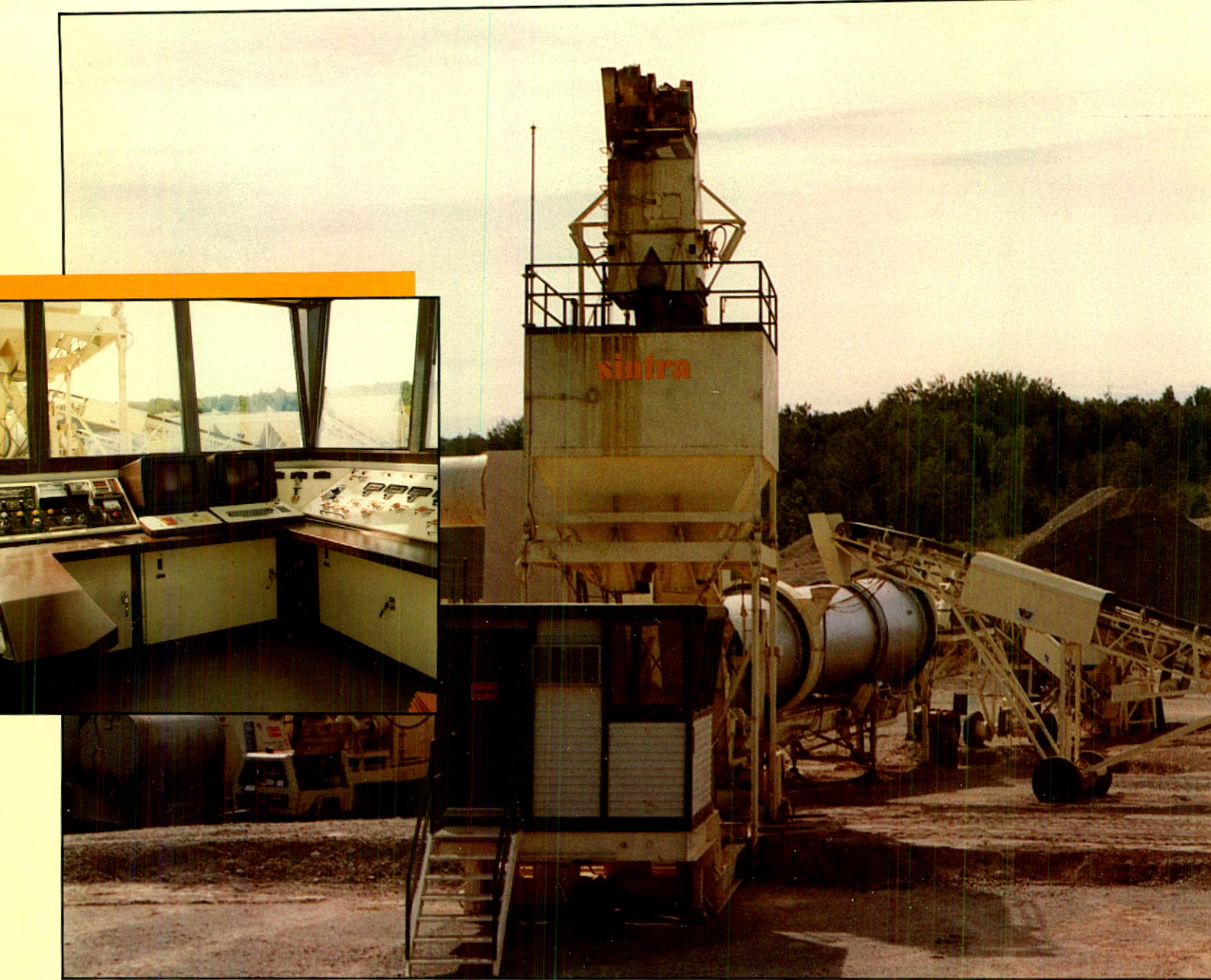
High technology: fully automatic drum-mix asphalt plant. Entirely fabricated in Montreal according to our own requirements.
