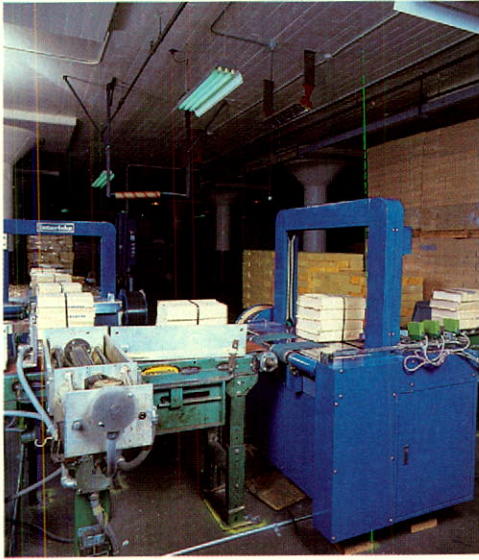
Automatic F20 plastic strapping machines bind Official Airline Guides for shipment at the Times Mirror Corporation's Los Angeles printing plant.
