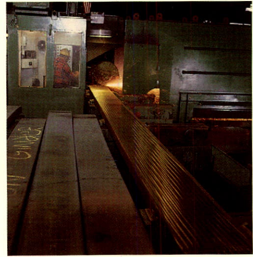
An automated slab grinder, purchased by Interlake in 1985, improves the surface quality of steel being processed for demanding customer applications.
