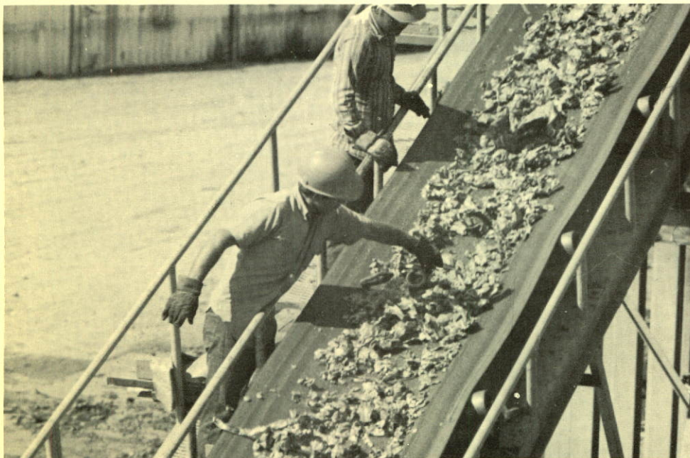
A complete auto body can be shredded into fist-size chunks of 'Intron' scrap in less than one minute. The Secondary Metals Division supplies processed raw materials to leading Canadian foundries and mills.
