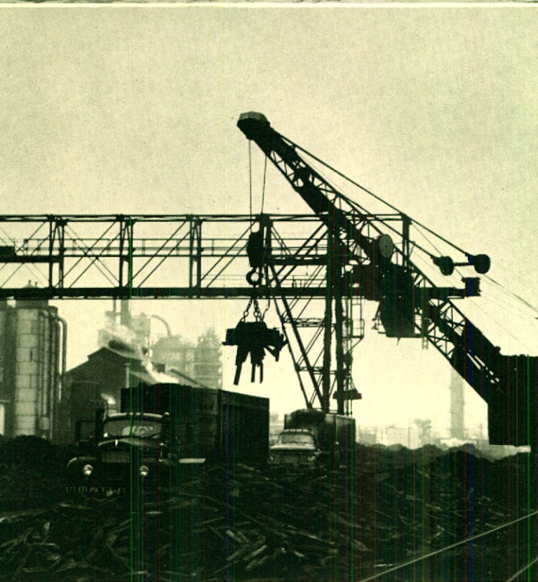
Above—Pelletized iron ore is unloaded at blast furnace dock. Below—Pig iron is loaded onto truck for delivery to customer.
