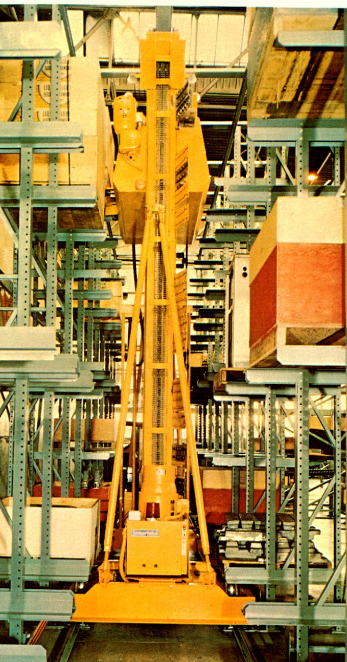
Interlake's new Courier, an automated pallet retrieval system, was introduced during the year. The first unit has already been sold.
