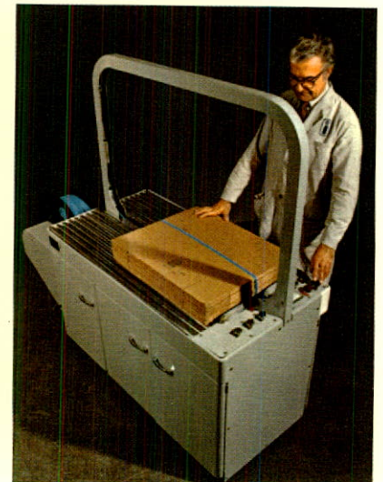
New in '69... this portable automatic machine applies nylon or polypropylene strap in many small packaging operations.
