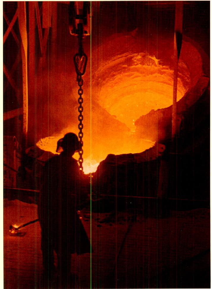
This Globe Division metallurgist is sampling a heat of ferroalloys at the Beverly, Ohio, plant, which includes the world's largest smelting furnace.
